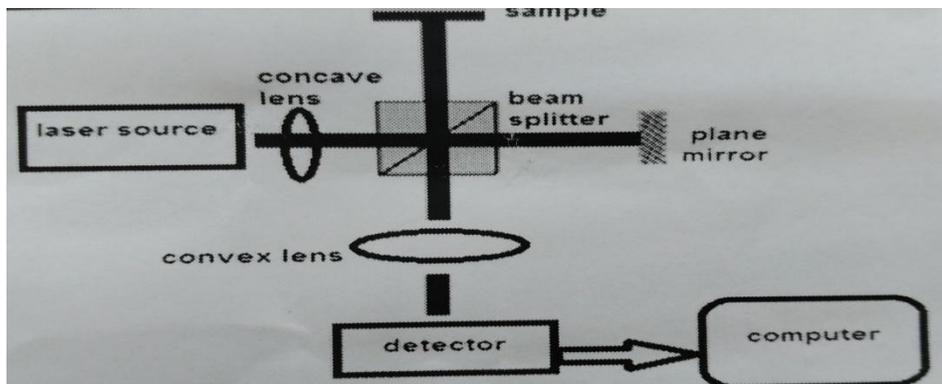
Figure (5) ,Rough surface ESPI setup.
