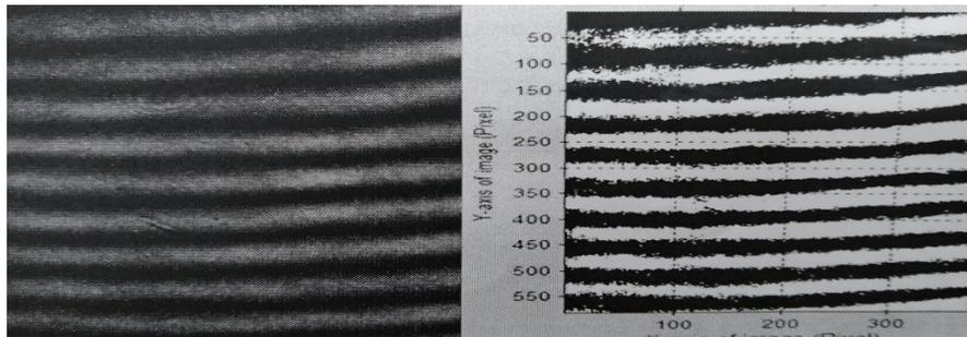
Figure( 9). Resulted image by ESPI technique for the displaced Ge sample and converted binary image for the same sample.
